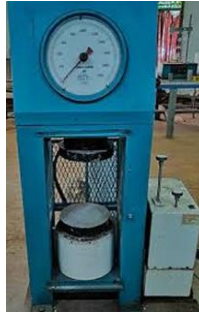
Figure 2. Compressive Strength Testing Equipment
